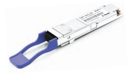
The Quad Small Form-factor Pluggable + (QSFP+) is defined by the MSA as a module capable of offering 4 independent transmit and receive channels each capable of 10Gb/s operation for an aggregate data rate of 40Gb/s. The QSFP+ also supports the Optical Transport Network (OTN).
