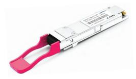
The Quad Small Form-factor Pluggable 28 (QSFP28) is defined by the MSA as a module capable of offering 4 independent transmit and receive channels each capable of 25Gb/s operation for an aggregate data rate of 100Gb/s. The QSFP28 also supports the Optical Transport Network (OTN).
