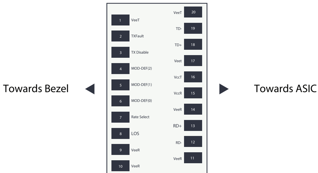
Figure 1. Diagram of host board connector block pin numbers and names
