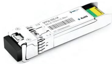
The Small Form-factor Pluggable 56 (SFP56) uses the PAM4 laser modulation offering a 53Gb Ethernet capability.
