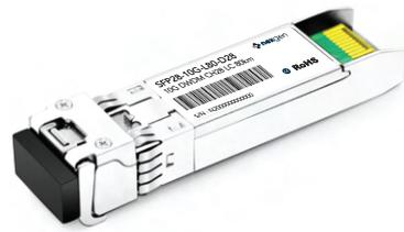
The **Small Form-factor Pluggable 28 (SFP28)** is defined by the MSA as having the the same form-factor specificities as the SFP+. The SFP28 port will typically be backwards compatible with SFP+ and supports 25/28Gb Ethernet, 32Gb Fiber Channel along with Optical Transport Network (OTN).
