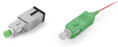
The Fiber Bragg Gratings (FBGs) come in various type (connectors, pigtail, patch cords,...) and are placed directly on the network fiber. When the light spectrum propagates through the FBG, only a specific wavelength called the “Bragg wavelength” is reflected, leaving the remaining wavelengths unaffected. By analyzing the Bragg wavelength behavior, defects on the fiber can easily be located.
