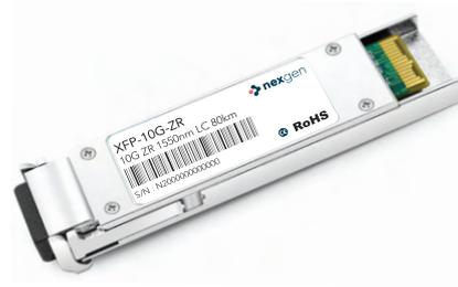
The “X” Form-factor Pluggable (XFP) Principal applications include 10 Gigabit Ethernet, 10 Gbit/s Fiber Channel, synchronous optical networking (SONET) at OC-192 rates, synchronous optical networking STM-64, 10 Gbit/s Optical Transport Network (OTN) OTU-2, and parallel optics links.
