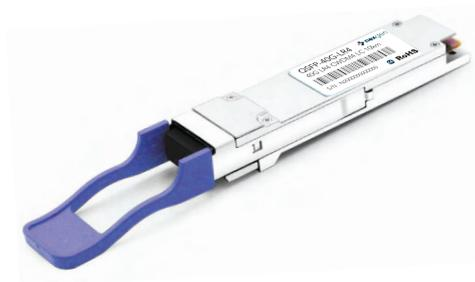
The **Quad Small Form-factor Pluggable + (QSFP+)** is defined by the MSA as a module capable of offering 4 independent transmit and receive channels each capable of 10Gb/s operation for an aggregate data rate of 40Gb/s. The QSFP+ also supports the Optical Transport Network (OTN).
